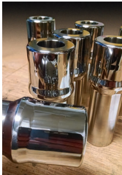
Before and After photos of an A2 component finished with 3 micron SC compound on a felt wheel
