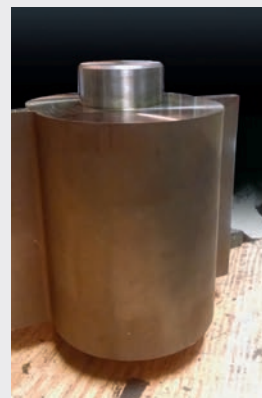
Before and After photos of an A2 component finished with 3 micron SC compound on a felt wheel
