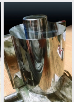
Before and After photos of an A2 component finished with 3 micron SC compound on a felt wheel
