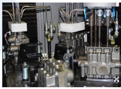
Simultaneous precision finishing and gauging of four bores in a hydraulic valve body.
