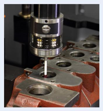
Automatic probing to find bore location and create machine offsets.
