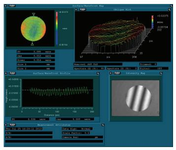
Interferogram of a sapphire wafer processed with the Engis Hyprez System exhibiting superior edge-to-edge flatness control with no edge roll-off.
