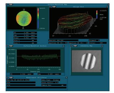
Interferogram of a sapphire wafer processed with the Engis Hyprez System exhibiting superior edge-to-edge flatness control with no edge roll-off.
