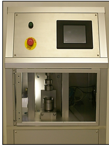
Fig. 12 – Crushing strength apparatus (US Patent 7,275,446)
